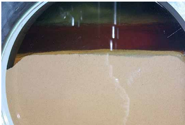
Fig. 5. Interface between water and 15% DS sugar solution above the resin bed.
